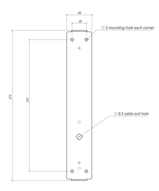
Backplates can be rotated 180 degrees- to allow cable exit to be positioned at top if required.
