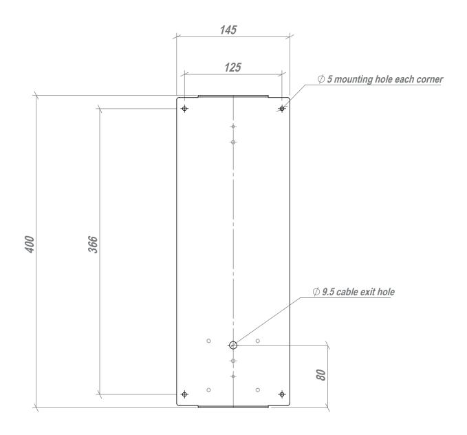
Backplates can be rotated 180 degrees- to allow cable exit to be positioned at top if required.
